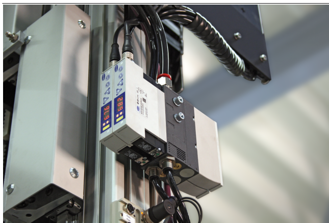
Central vacuum generation by compact ejectors SMPi
